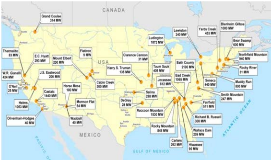
Figure 3-6 Pumped-hydro storage facilities in the US (Source: HDR)
